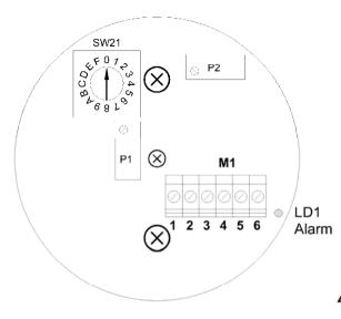
**SW21**: Rotative switch to regulate the alarm threshold
